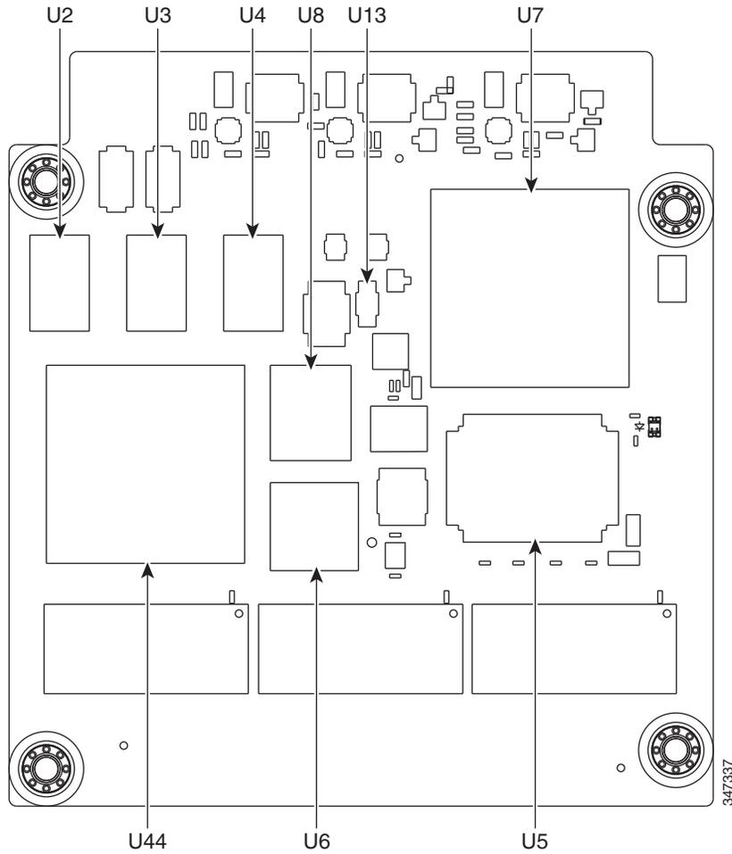
**Table 15** Thermal Details for the Thermally Significant Components of Cisco ESS 2020 (Main Card)
