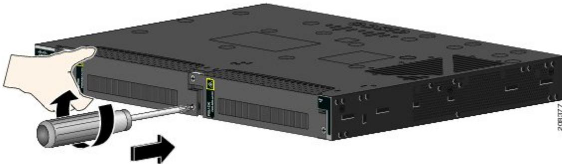
**Step 7** Use a ratcheting torque screwdriver to torque each screw to 8–10 in-lb.
