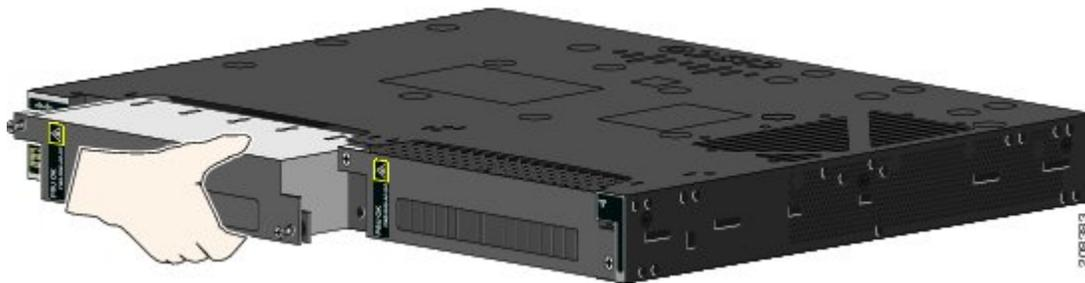
**Step 3** Insert the power-supply module into the slot, and gently push it in.
