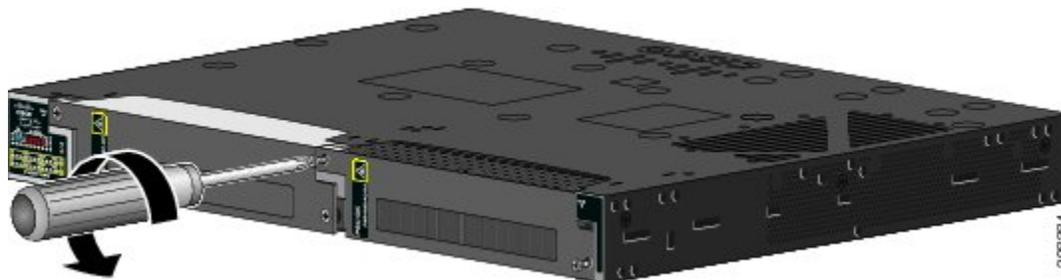
**Step 4** Remove the power-supply module from the power slot. The power-supply module might be hot. See the following figure.
